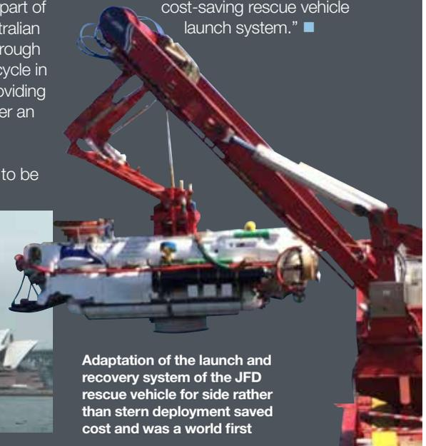
Adaptation of the launch and recovery system of the JFD rescue vehicle for side rather than stern deployment saved cost and was a world first
